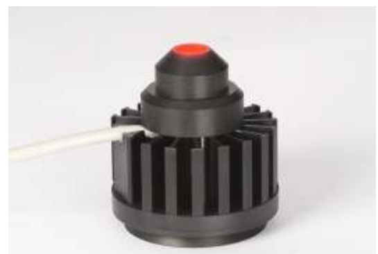
The ultra-fast color MetaLED illumination is utilized to acquire high quality true color images with a monochrome camera.
