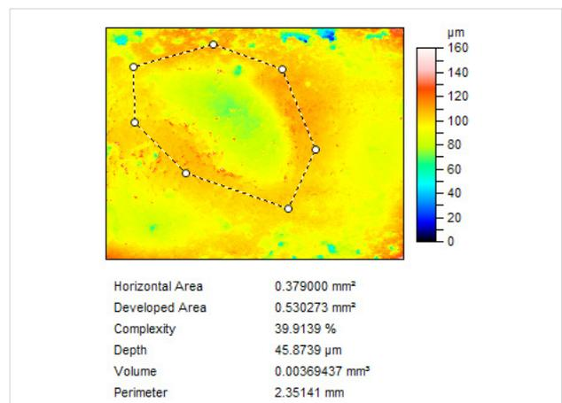
Figure 5c Height map after form removal by a polynomial of order 4, parameters are obtained with the tool "measurement of a wrinkle"
