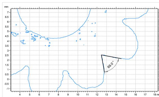
Figure 3 The angle between adjacent teeth of the gear wheel is measured in the horizontal contour.
