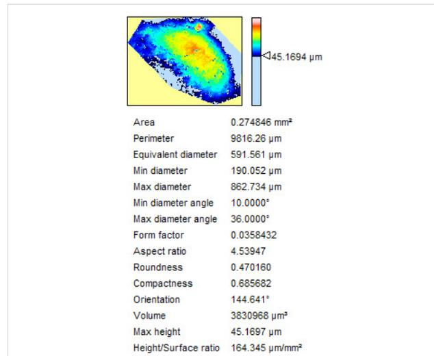
Figure 5b Measurement of wear volume and other geometrical parameters of the defect by the tool "volume of island"
