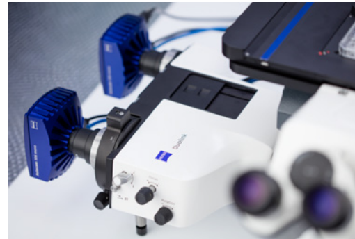
Use Duolink and ZEN imaging software to perform high speed imaging with two spectrally separated channels simultaneously.
