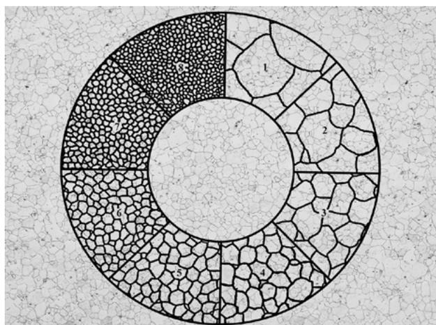
**Figure 2** Non-alloy, low-carbon steel of high purity. Above: Steel microstructure, showing ferrite grains. Below: grain size comparative overlay as per ASTM E112. Etching: 1% HNO<sub>3</sub>. 100× magnification. (Objective: EC Epiplan-NEOFLUAR 10×/0.25 DIC; brightfield)
