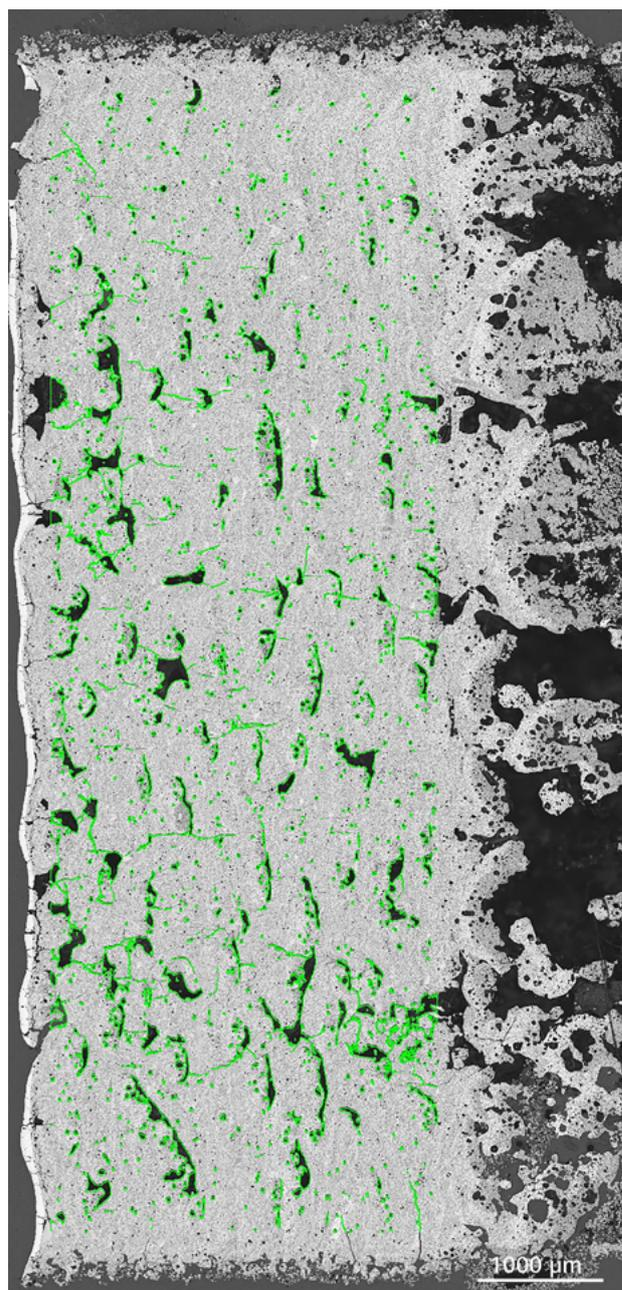
**Figure 8** Laser-fused component made of metal. Production-dependent porosity allows conclusions to be made about the production parameters. Unetched. 100× magnification. Consolidated image. (Objectives: EC Epiplan-NEOFLUAR 20×/0.50 HD DIC, brightfield) Tile Image (8×6)
