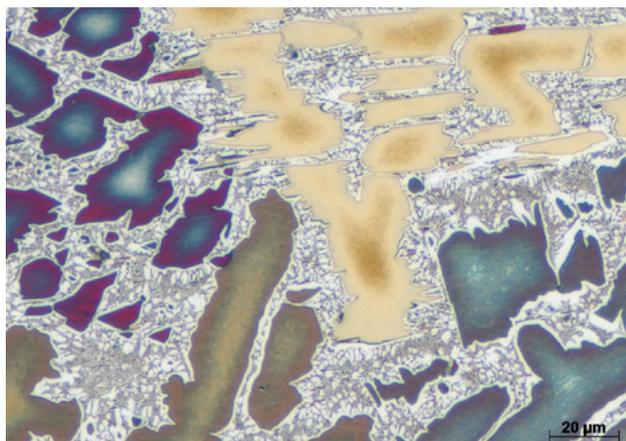
**Figure 4** Bell bronze; dendritic  $\alpha$ -mixed crystals in different crystal orientations;  $\alpha+\delta$ -eutectoid in remaining fields.
