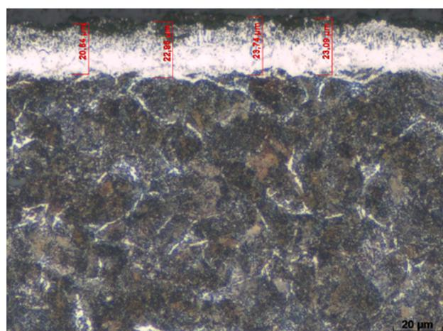
**Figure 3** TENIFER® nitrided case; compound layer (25 μm) and diffusion layer (320 μm). Matrix: heat-treated structure made of tempered martensite with individual nitride deposits. Etching: 3% HNO<sub>3</sub>. Above, 50× and below, 500× magnification. (Above: objective: EC Epiplan-NEOFLUAR 5×/0.14; below: objective: EC Epiplan-NEOFLUAR 50×/0.55 HD DIC, brightfield)
