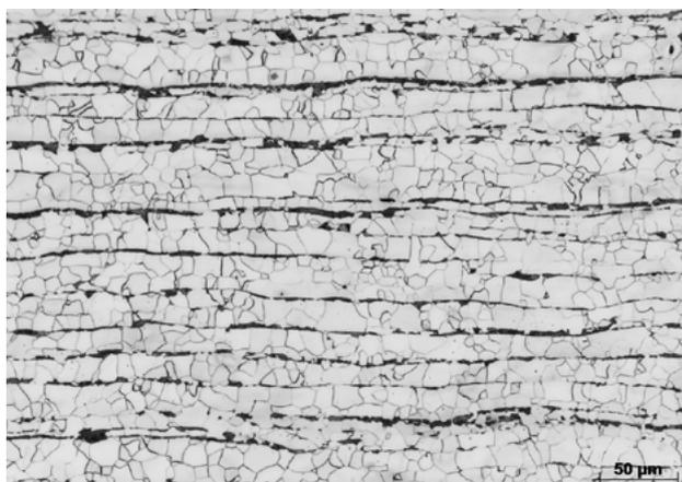
**Figure 6** Longitudinal section of structural steel. Formed banded structure made of ferrite (bright) and perlite (dark) due to normalized rolling. Etching: electrolytically etched with A2. 200× magnification. (Objectives: EC Epiplan-NEOFLUAR 20×/0.50 HD DIC, brightfield)
