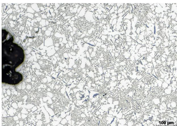
**Figure 7** Aluminum silicon cast alloy; hypoeutectic alloy with microshrinkage and micropores. Points of varying fine and coarse formations of eutectic. Unetched. Consolidated image. Top: 100× magnification taken with Tile Image; Bottom: 100× magnification. (Objective: EC Epiplan-NEOFLUAR 20×/0.50 HD DIC, brightfield)
