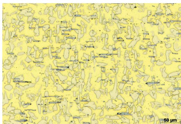
**Figure 5** Special brass: matrix of  $\beta$ -mixed crystal with oriented  $\alpha$ -crystals. Silicide precipitation structure oriented in rolling direction.
